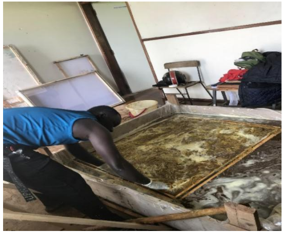
Figure 15: Mould and deckle dip to scoop set fibre using for board
