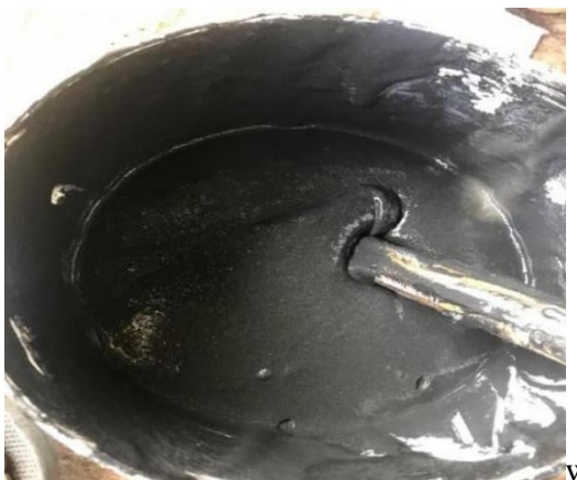
Figure 20: Procedure of making matt from charcoal and how matt is added onto the surface of the soft board to produce the blackboard.
