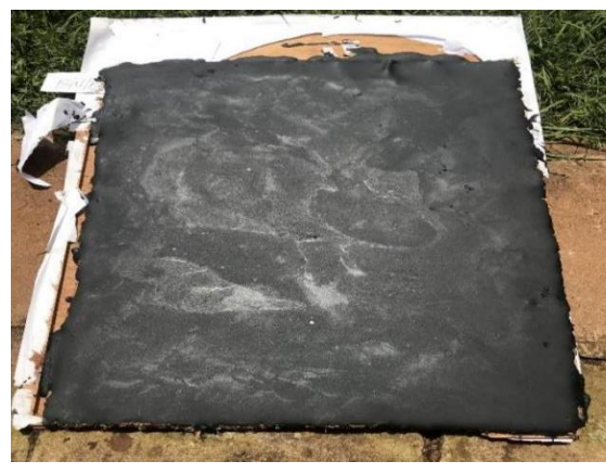
Figure 20: Procedure of making matt from charcoal and how matt is added onto the surface of the soft board to produce the blackboard.
