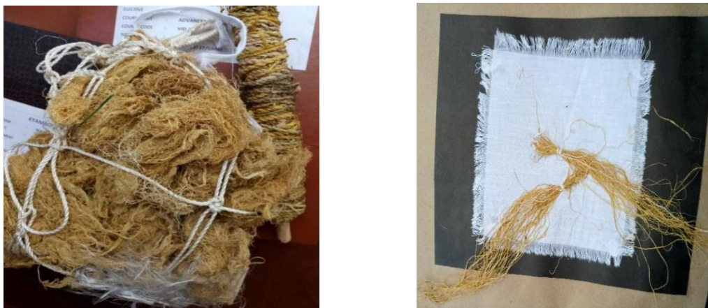
Figure 10: Processed fibres from maize husk for weaving.
