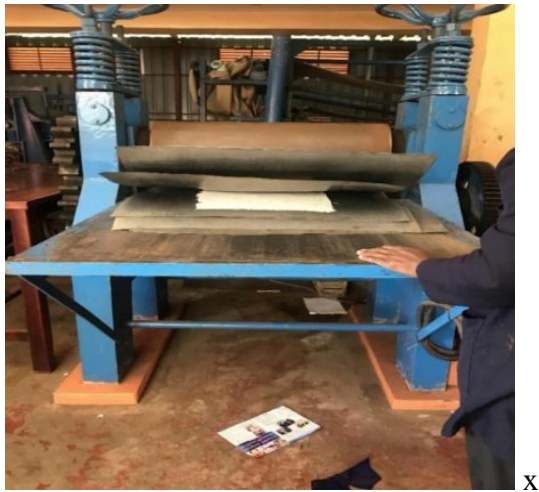
Figure 26: Calendaring operated to press paper and Pile paper for making books. Source: Photo by the researcher
