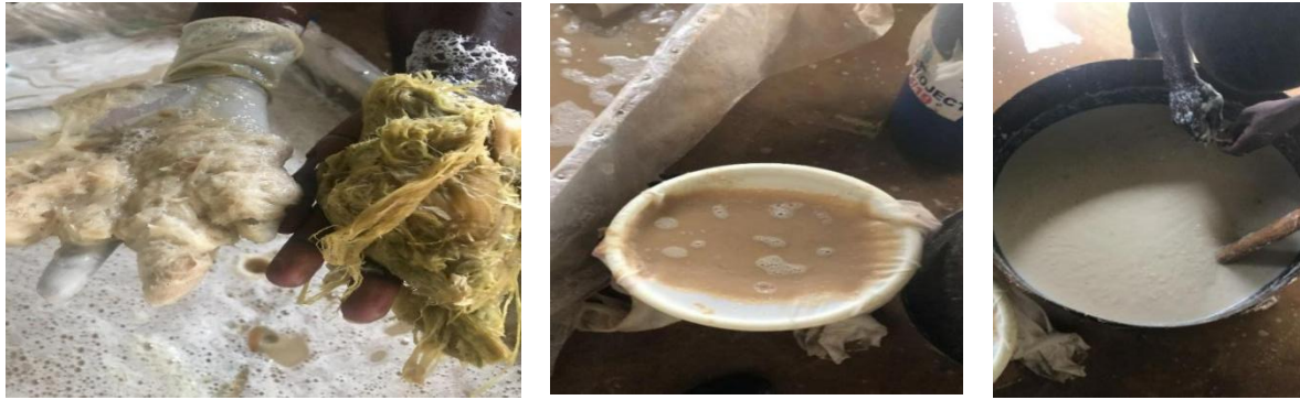
Figure 23: Bleached fibre and unbleached fibre (m), Scoop pulps freshening pulps for bleaching and picking the unbroken fibre (n), and bleached pulps ready for papermaking (o).
