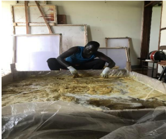
Figure 15: Mould and deckle dip to scoop set fibre using for board
