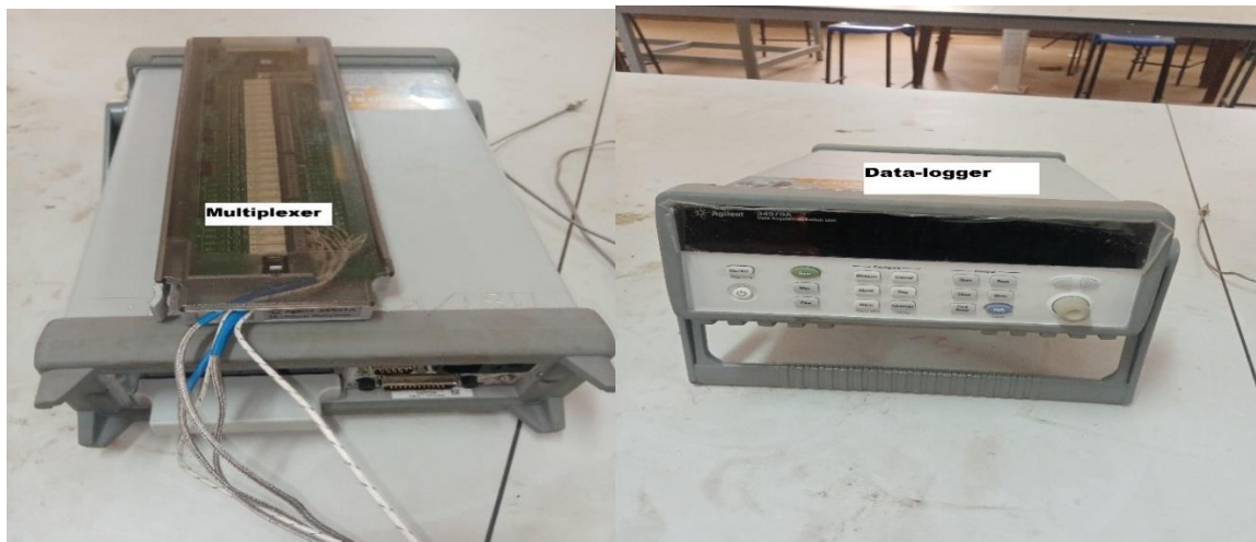
Figure 3.8: The 20-channel multiplexer and the data logger.
