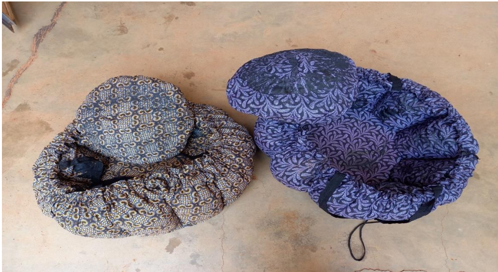
Figure 3.3: A photograph showing the insulating wonderbag used for heat retention cooking experiment.
