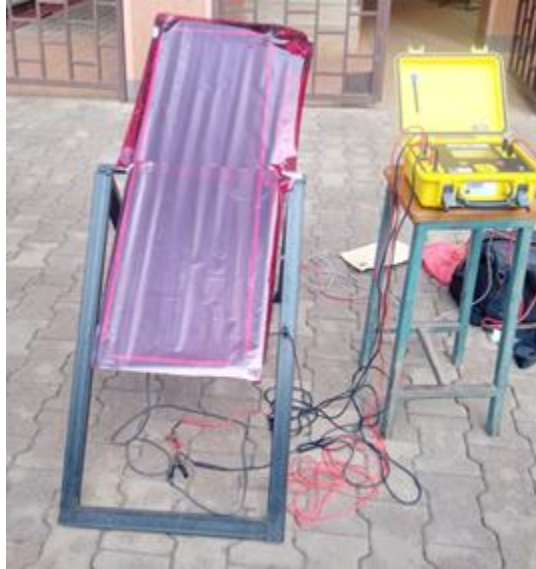
Figure 3. 3: The I-V tracer and amorphous module with red filter.
