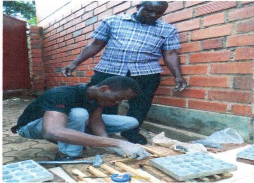
Figure 4.12: Researcher and one of the students setting up moulds and pallets to be used in moulding of the briquettes (2016).
