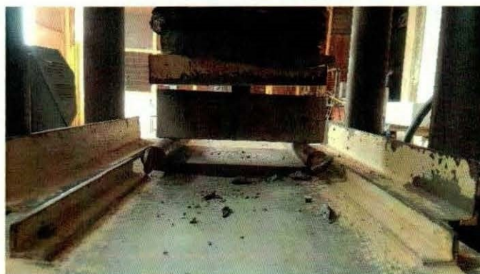
Figure 3.8: Test setup for Flexural strength test
