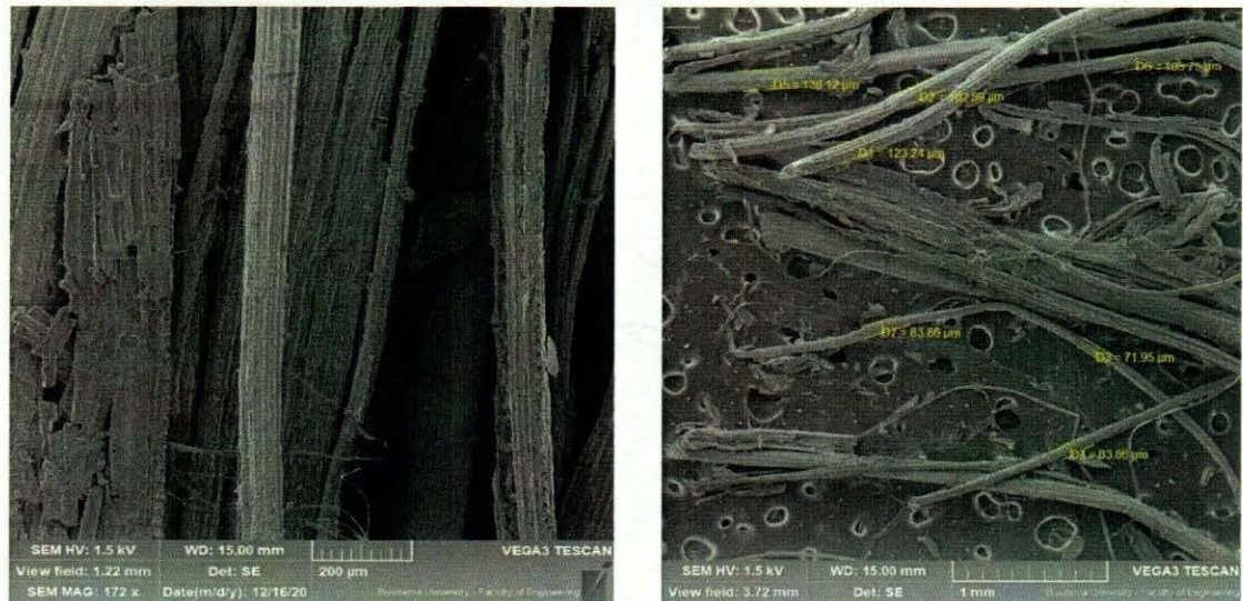
Figure 4.1: SEM Micrographs-Banana Fibre Microstructure and Fibre Diameter
