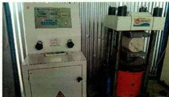
Figure 3.7: Test for Split tensile strength
