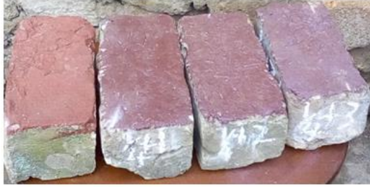
Application of manufactured ferric oxide paint on surfaces
