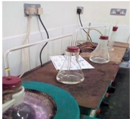
Ferric oxide heated on a round bottomed hot plate (mantle)
