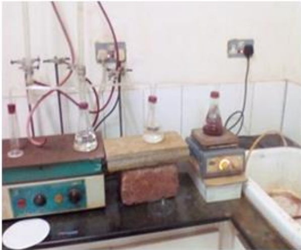
Ferric oxide heated on a flat hot plate
