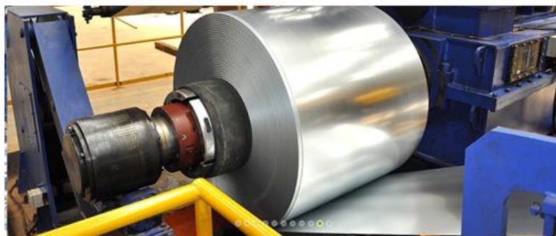
(b) A pickled Steel Coil being removed from the Pickling Line
