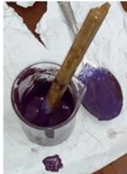
Mixing ferric oxide with glaze forms Violet colour
