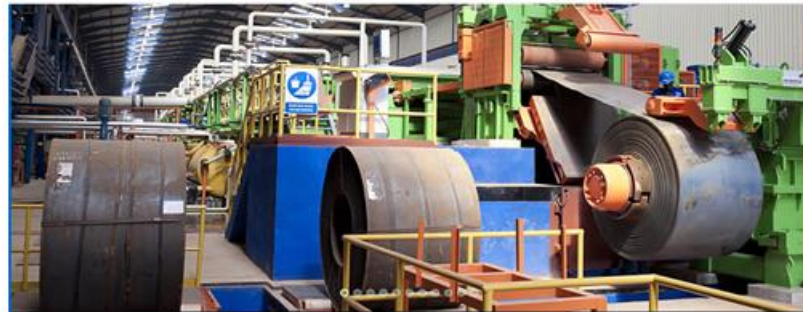
(a) A Steel Coil being loaded on the Pickling Line
